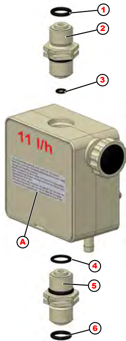
Fig. 19: Replace the suction / pressure valve and metering cartridge
